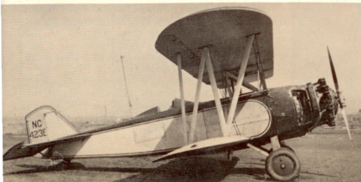
The Boeing Model 95 of 1929, with 525 h.p. Pratt and Whitney Hornet engine, reverted to large size and high power for mail and express on the trunk lines. It was the last of the big single-seat biplanes. Span is 44 feet, 3 inches; length, 31 feet, 11 inches; gross weight, 5,840 pounds; and cruising speed is 120 m.p.h. with 1,600 pounds payload.
